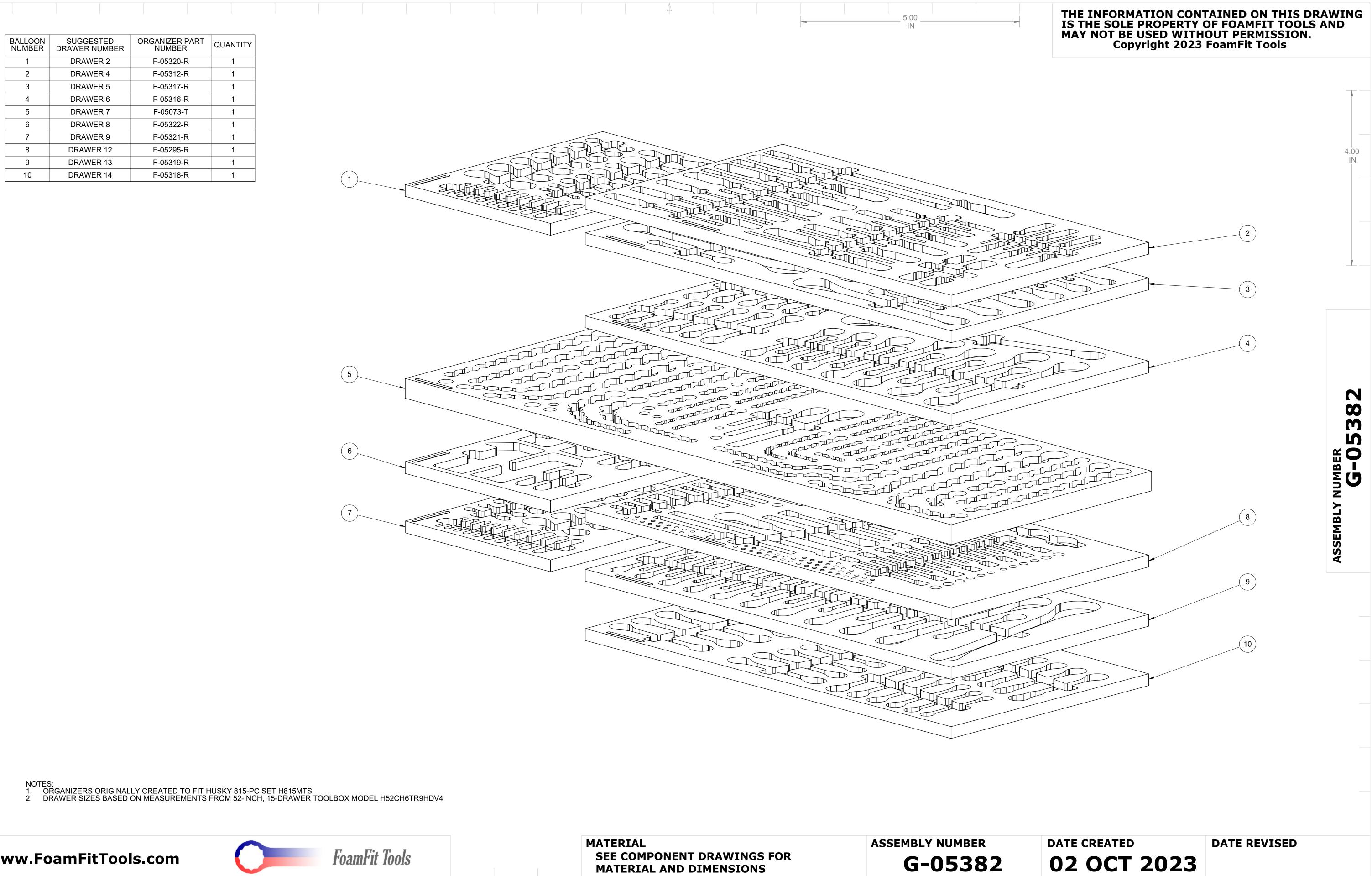
NOTES: 1. ORGANIZERS ORIGINALLY CREATED TO FIT HUSKY 815-PC SET H815MTS 2. DRAWER SIZES BASED ON MEASUREMENTS FROM 52-INCH, 15-DRAWER TOOLBOX MODEL H52CH6TR9HDV4
