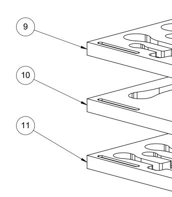
NOTES: 1. ORGANIZERS ORIGINALLY CREATED TO FIT HUSKY 1025-PC SET H1025MTS 2. DRAWER SIZES BASED ON MEASUREMENTS FROM 56-INCH, 23-DRAWER TOOLBOX MODEL HOTC5623BB2S
