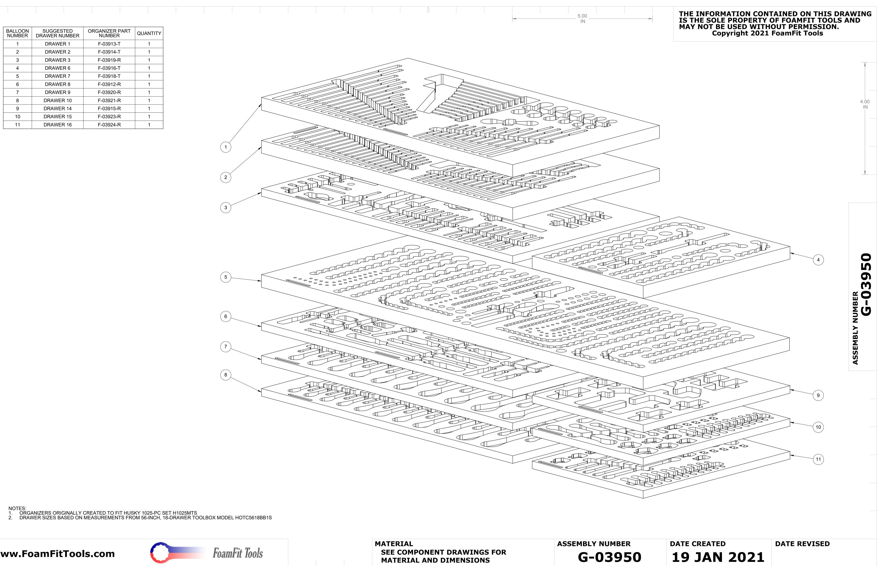
NOTES: 1. ORGANIZERS ORIGINALLY CREATED TO FIT HUSKY 1025-PC SET H1025MTS 2. DRAWER SIZES BASED ON MEASUREMENTS FROM 56-INCH, 18-DRAWER TOOLBOX MODEL HOTC5618BB1S
