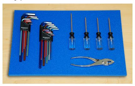
Use a marker to trace the tools. We used a liquid chalk marker as shown, but neon dry-erase markers also work well.
